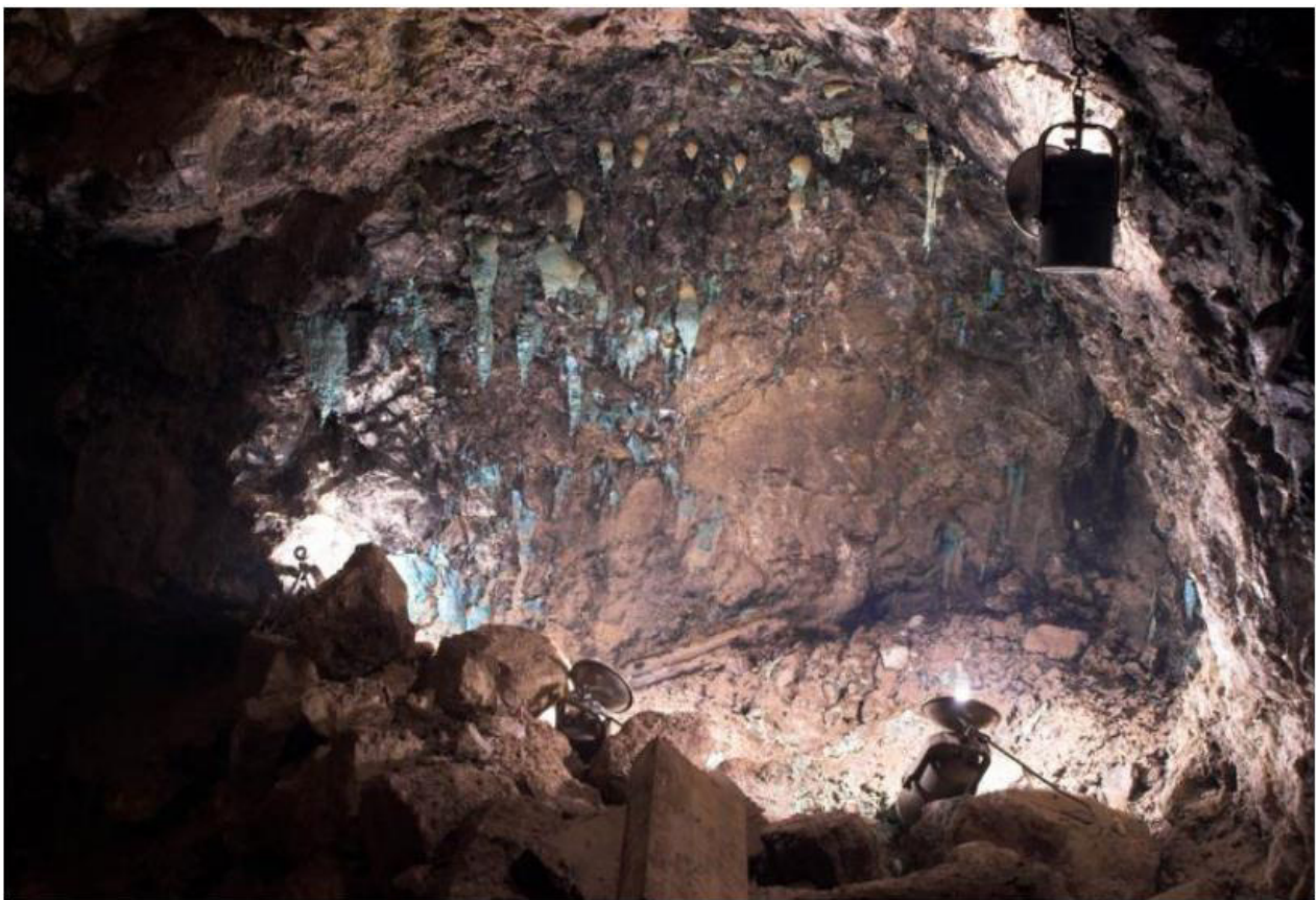
Green Vault: Secondary copper minerals (malachite, brochantite, chrysocolla) formed by the oxidation of copper ores in the quartz veins of the Suggental silver mine ( mine website )
